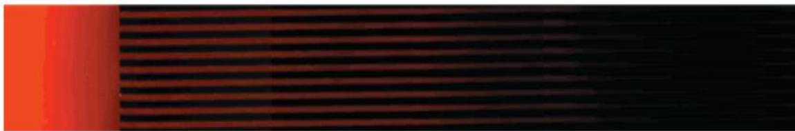
Figure 11 Continuous gradients of protein (rabbit IgG) produced using high aspect ratio \mu FNs on a PDMS surface [23].
